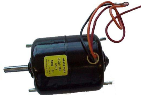
GR314 CW ROTATION GR315 CCW ROTATION 3" BODY, 5/16" SHAFT 2 SPEED
